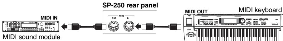
To connect the SP-250 to a computer, you need a MIDI interface for the computer, sequencing or musical notation software, and two standard MIDI cables. Connect
