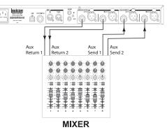
This setup lets the MX300 act as two effects processors. Separate input sources are fed into the MX300 and processed independently with different effects, then output as separate mono signals. The **Input Source** must be set to **Anlg Stereo** in the System menu (described on page 30). This setup is ideal for programs using the Mono Split routing (see page 16 for more information about routings).
