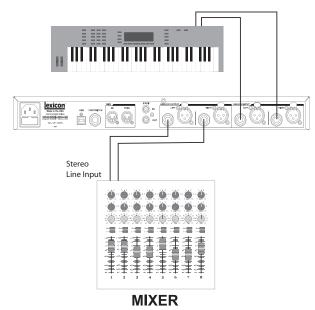
This setup allows a line level instrument such as an electronic keyboard to be connected directly to the MX300. Connect the outputs of the line level instrument to the MX300 inputs and connect the MX300 outputs to the input channels of a mixer, or the inputs of a powered speaker system. The **Input Source** must be set to **Anlg Stereo** in
