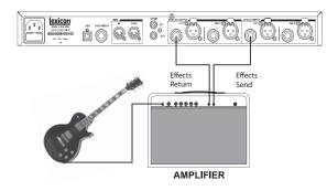
This setup is optimized for use within a guitar amplifier effects loop system. A single input source is fed into the MX300 and output as a mono signal. The **Input Source** must be set to **Anlg Mono L** in the System menu (described on page 30). This setup is ideal for programs using Cascade, Parallel, and Stereo routings (see page 16 for more information about routings).
