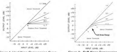
Figure 1: Hard Knee Compression Curve
