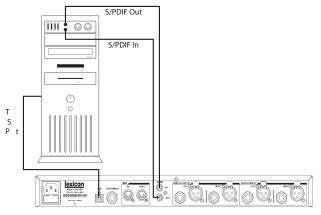
This setup is ideal if you are using the MX300 as a hardware plug-in in a digital recording system. This setup requires that you are using an I/O device with S/PDIF In/Out, or a digital mixer with S/PDIF I/O option. The **Input Source** must be set to **Digital**, and the **Clock Source** should be set to **Digital** in the System menu (described on pages 30-31).
