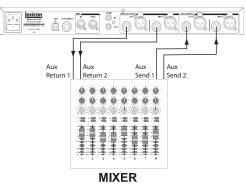
This setup lets the MX300 act as two effects processors. Separate input sources are fed into the MX300 and processed independently with different effects, then output as a mixed stereo signal. The **Input Source** must be set to **Anlg Stereo** in the System menu (described on page 30). This setup is ideal for programs using the Mono Split routing (see page 16 for more information about routings).
