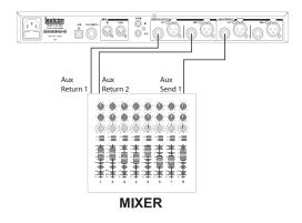
This setup is the most commonly used configuration in both live and studio applications. A single input source is fed into the MX300, processed, and output as a stereo signal. The **Input Source** must be set to **Anig Mono L** in the System menu (described on page 30). This setup is ideal for programs using Cascade, Parallel, and Stereo routings (see page 16 for more information about routings).
