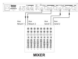
Stereo Mode configures the MX300 as a single stereo input/output processor. Left and Right signal separation is maintained through the effects chain. The **Input Source** must be set to **Anlg Stereo** in the System menu (described on page 30). This setup is ideal for use with programs using Cascade, Parallel, and Stereo routings (see page 16 for more information about routings).
