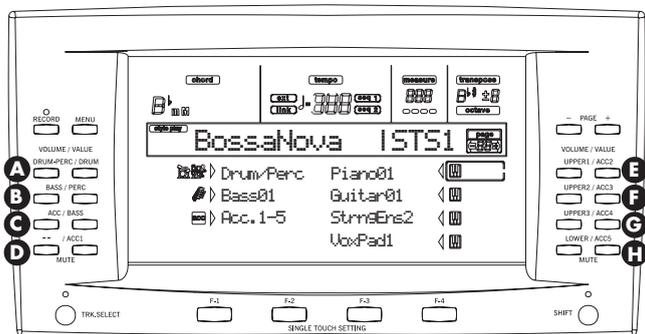
A corresponding track name is printed over each button pair. These names show the corresponding track the button pair affects in the main page of the Style Play mode.
