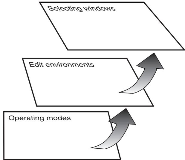
**Operating modes.** (See diagram at the bottom of this page). At the lowest level, an operating mode is always active. The current operating mode is indicated by the lit LED on the STYLE PLAY, B.SEQ, SONG PLAY, SONG or PROGRAM button in the MODE section. The relevant icon lights up in the display.
