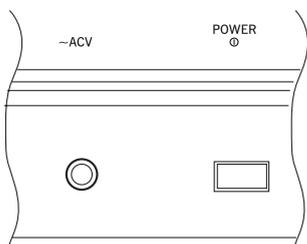
Connect the supplied AC power adapter to the dedicated socket on the rear of the instrument. Then, plug it into a wall socket.
