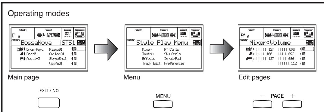
**Edit environment.** (See diagram at the bottom of this page). When you press GLOBAL or DISK, an edit environment overlaps the current operating mode. Press EXIT to go back to the current operating mode.
