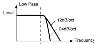
This is a filter that cuts the high-frequency region above the cutoff frequency. □
