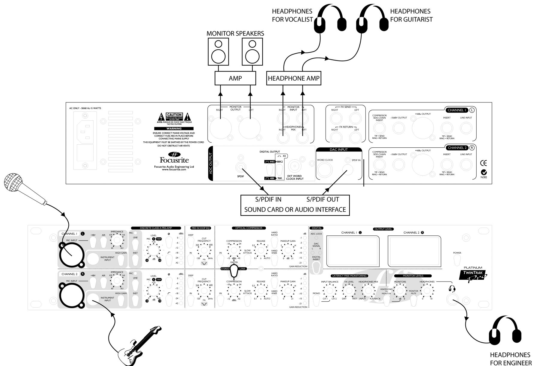
**STEREO RECORDING (COINCIDENT PAIR) WITH DIGITAL MONITORING**
