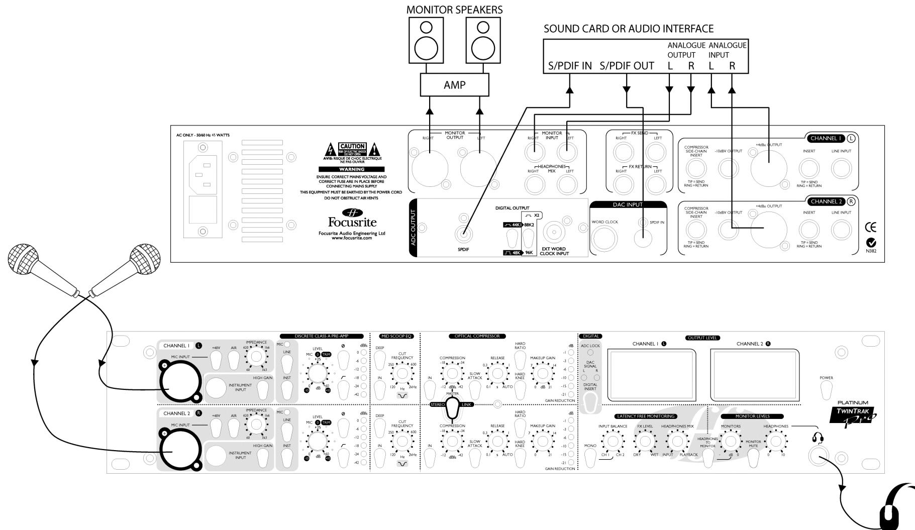
**DIGITAL INSERT FOR STEREO COMPRESSION AND MASTERING, PLUS COMPRESSOR SIDECHAIN INSERT FOR FREQUENCY-SELECTIVE COMPRESSION**
