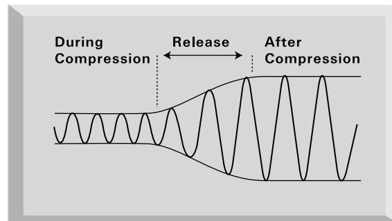
Short release times mean the compressor very quickly returns the signal to its normal level. This can produce a ‘pumping’ sound, where the changes in volume are very audible. Depending on the style of music, this can be undesirable, or a useful creative effect.
