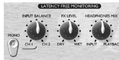
The LATENCY FREE MONITORING section is used in conjunction with the MONITOR LEVELS section to provide flexible monitoring of both the signal being recorded and an existing stereo mix.
