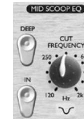
**IN (switch)** - Switches the MID SCOOP EQ into the signal path. When engaged, the red LED in the switch cap is lit.
