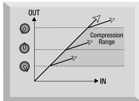
The amount by which the compressor reduces the gain is determined by the 'ratio'. The ratio is conventionally expressed as a numerical value, e.g. '4:1', which represents the amount by which the gain is reduced when the volume of the signal rises above the threshold.
