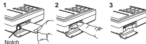
To remove the card, press it all the way to the back of the slot to unlock it, and then pull out the card.
