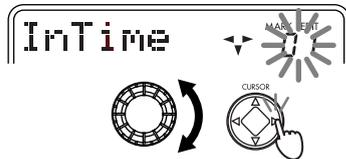
**note** By pressing the [CURSOR] down key, you can edit the time location of the selected mark. You can also press the [PLAY] key to play back the sound for approximately two seconds from the selected time location.
