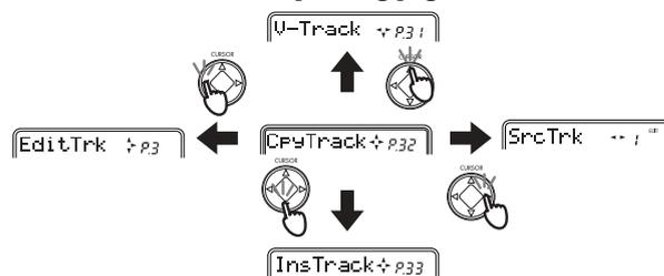
**note** By continuing to hold down the mode key you pressed, you can move through the pages after entering the mode in the same way as by pressing the [CURSOR] down key.
